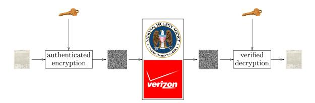
Bob receives the ciphertext and uses the secret key to **decrypt** the ciphertext, computing the original plaintext. Subsequent messages from Alice to Bob (or from Bob to Alice) are encrypted and decrypted similarly.
